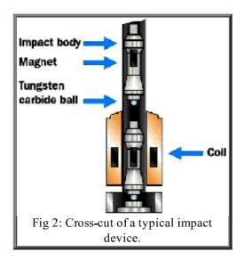
The inventor of this method, D. Leeb, defined "his own" hardness value, the Leeb hardness value. The Leeb hardness value, HL, is calculated from the ratio of the impact and rebound speed according to:
