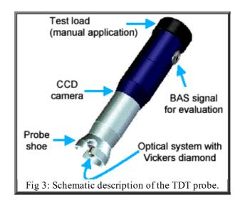
By applying a certain test load (e.g. 50 N) the diamond penetrates into the material. The indentation size of the Vickers diamond, i. e. the lengths of the diagonals, is automatically measured under load by viewing through the diamond with an optical system having a CCD camera. Data evaluation is then made in the instrument. As Vickers hardness is simply defined
