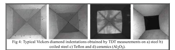
Figure 4 shows some typical Vickers diamond indentations obtained by the TDT instrument on different materials under test. TDT – for example – allows to determine the hardness of bulk material
