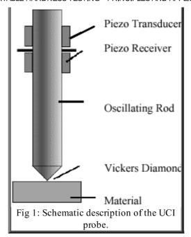
When the test load is applied, a frequency shift occurs as the diamond penetrates into the material. This frequency shift will become greater when the test indentation becomes larger, that means when the diamond penetrates deeper into "soft" material. Analogously, the smallest frequency shift is produced by hard test materials; the diamond penetrates only slightly into the material and leaves a small indentation.
